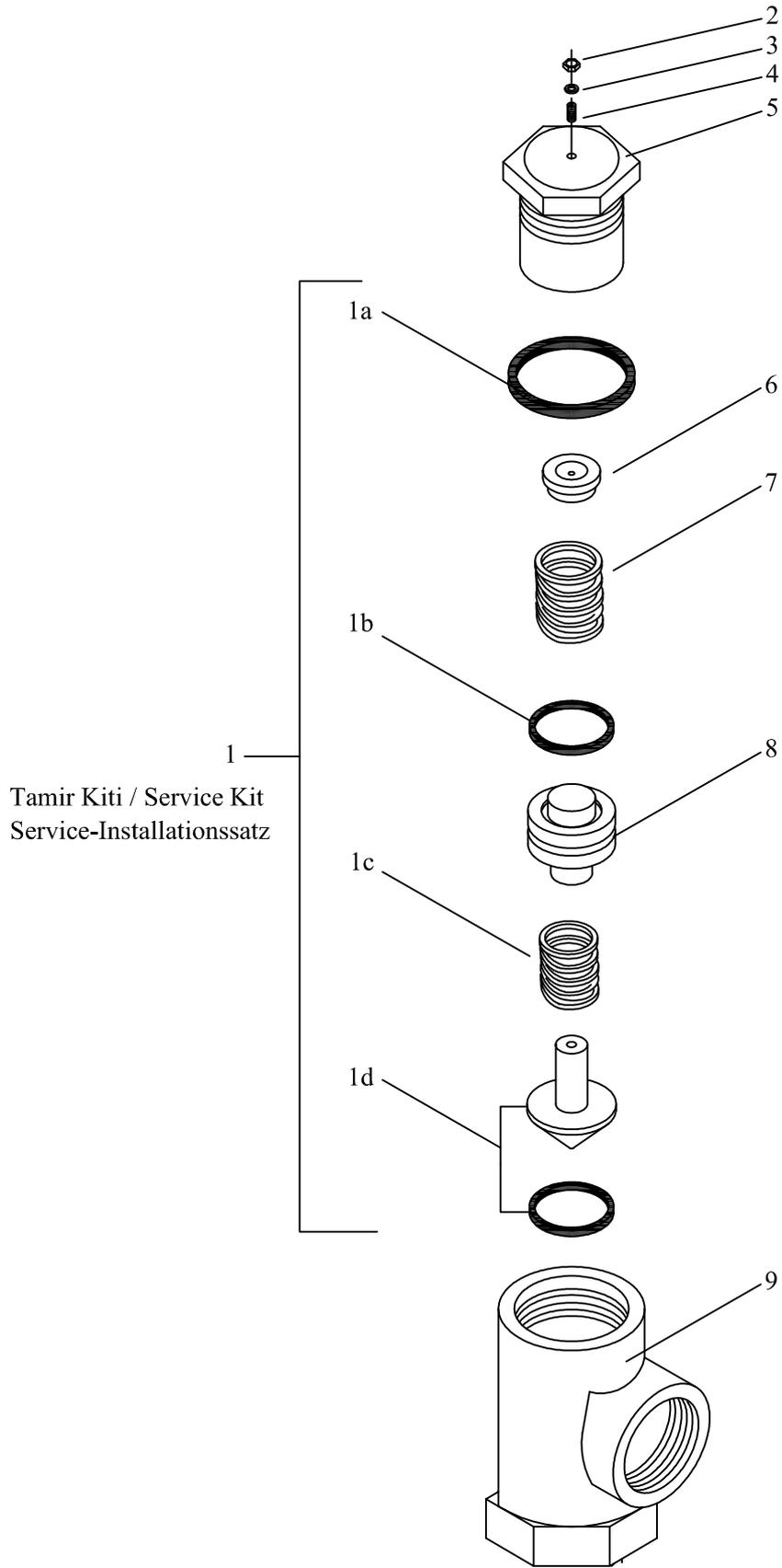
**MINIMUM BASINÇ VALFİ / MINIMUM PRESSURE VALVE / MINDESTDRUCKVENTIL (218951-1)**
